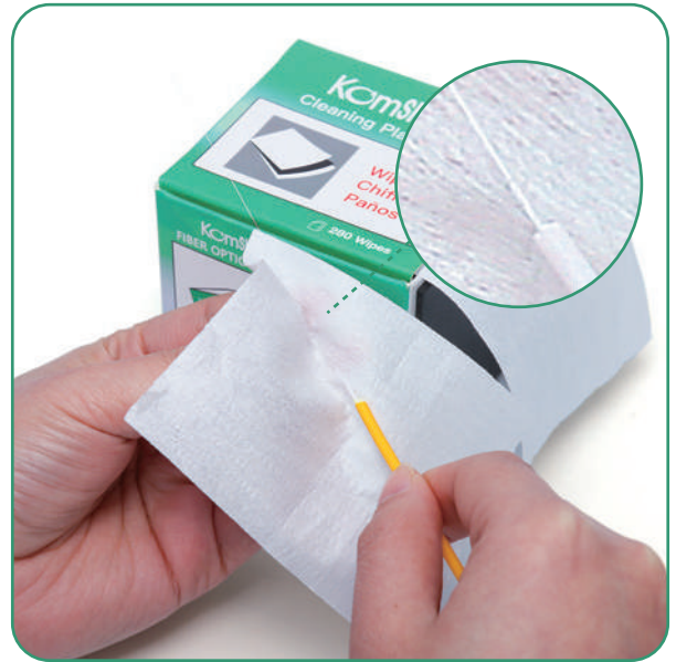
Direct wiping of bare optical fibers
